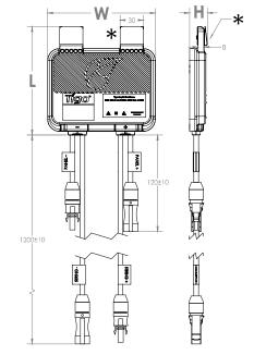
\*Clips can be removed for rack mounting Module frame specifications for mounting TS4-A
